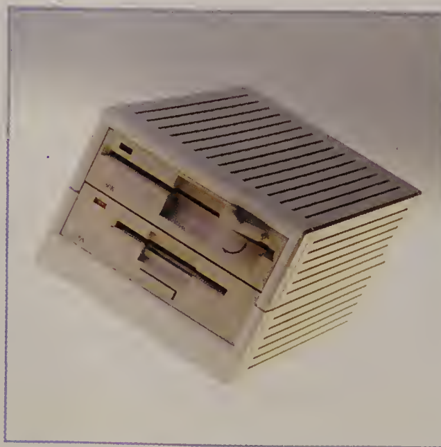
One possible DaynaFile configuration would include two drives—a 5¼-inch 360K drive and a 3½-inch 720K drive.
